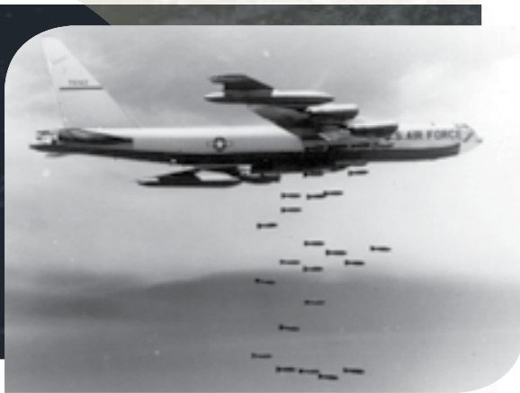
1965/1966 A U.S. Air Force Boeing B-52F-70-BW Stratofortress (s/n 57-0162, nicknamed "Casper The Friendly Ghost") from the 320 th Bomb Wing dropping M117 750 lb (340 kg) bombs over Vietnam. This aircraft was the first B-52F used to test conventional bombing in 1964, and later dropped the 50,000th bomb of the "Arc Light" campaign. B-52Fs could carry 51 bombs and served in Vietnam from June 1965 to April 1966 when they were replaced by B-52Ds which could carry 108 bombs.
